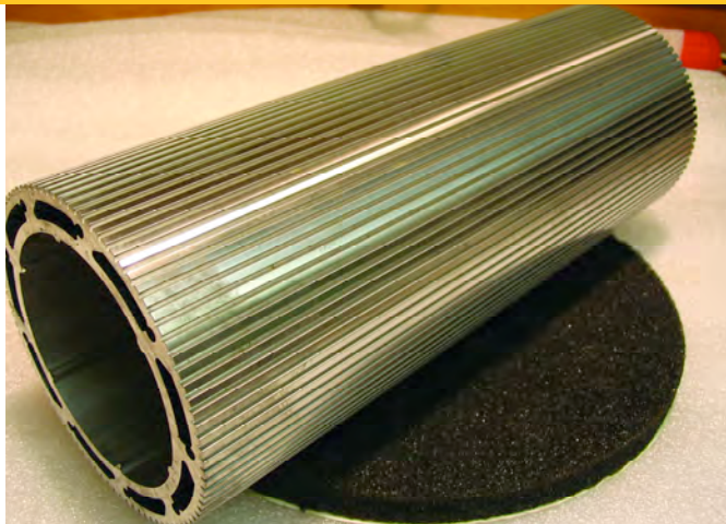
Aluminum Idler Roll: Sample part sent to Ultrasonic Power Corporation to test clean in their lab. The complementary service will determine if ultrasonic cleaning is suitable for an application. Images courtesy of Ultrasonic Power Corporation.
