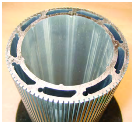
Aluminum Idler Roll after five minute test cleaning using a BT 90H and Brulin 815GD at a 10 percent mixture and a temperature of 140° F.
