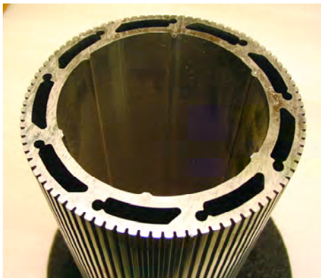
Aluminum Idler Roll before cleaning.
