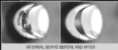
INTERNAL BURRS BEFORE AND AFTER
